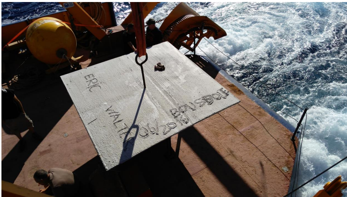
Picture of the dead weight on the deck of the “Castor 02” vessel, ready to be deployed at BOUSSOLE.
